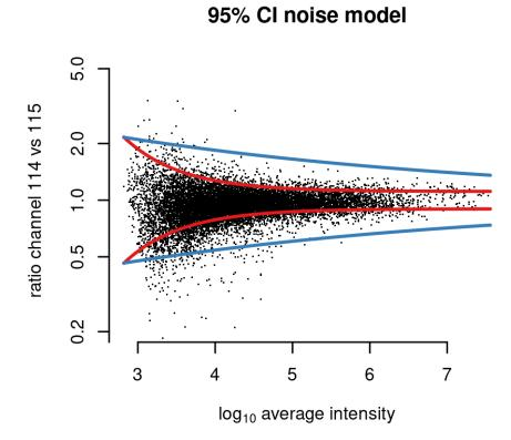
Figure 3: Red lines denote the 95 % confidence interval as estimated by the noise model on background proteins. The blue line is estimated as non 1:1 noise model based on only spectra of CERU proteins.
