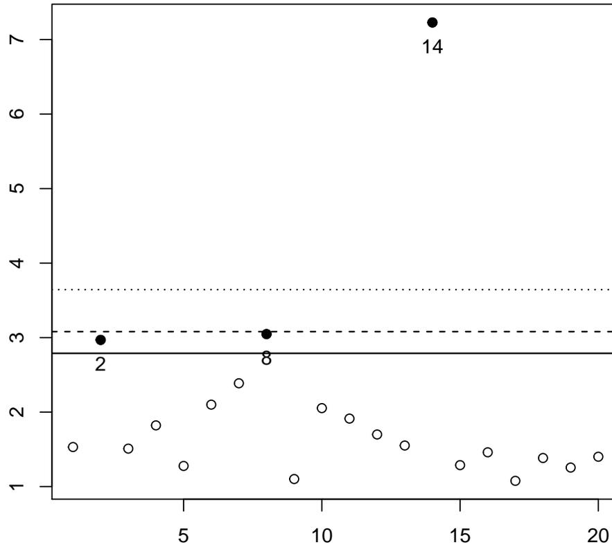
Figure 4: Results of MDQC using the global PCA method. The MDs (y-axis) are computed on the first four principal components for each array (x-axis). The solid, dashed and dotted lines indicate the square root of the 90th, 95th and 99th percentile of the Chi-Squared distribution, respectively. Outlying arrays are identified using solid points.
