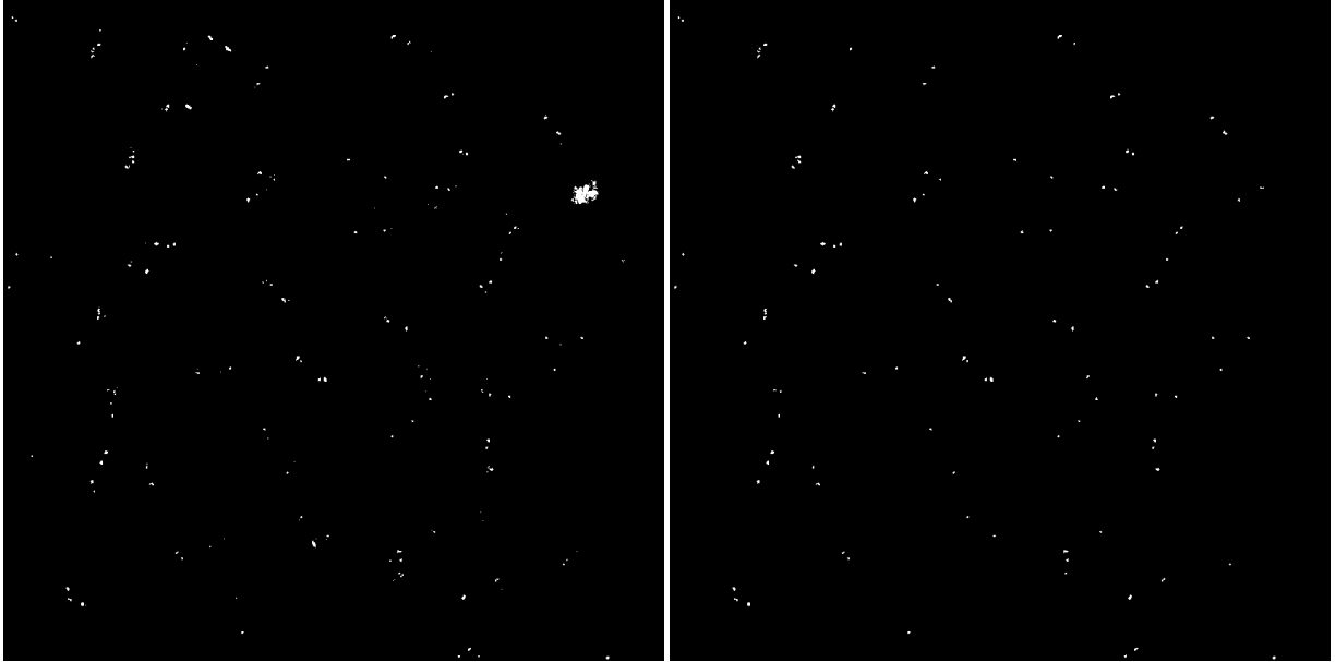
Figure 3. The original input image is given on the left side. Applying analyseParticles with MinSize=5 and MaxSize=20 results in the image shown on the right side. Components smaller than 5 pixels and larger than 20 pixels have been removed.
